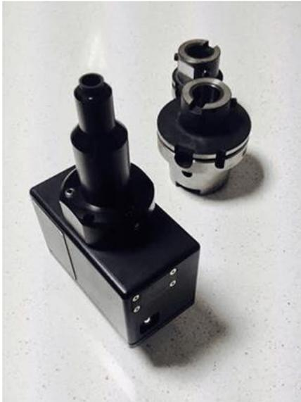
The **MEPULS**® system is an ultrasonic thickness measurement sensor integrated in machine tools to perform measurement campaigns automatically without interrupting the machining cycle. The capabilities of this innovative system range from production control to qualification of parts directly on the machine. It will also assist you in the automated phases of thickness control for re-machining.
